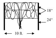
For trailing varieties and raspberry plants, you will need a trellis. To construct a simple trellis use two 7-8 feet upright posts sunk 2 feet in the ground leaving 5-6 feet above ground. Anchor end posts. Attach three 9-gauge wires at 18-inch intervals beginning 24 inches from the ground. Place posts no more than 20 feet apart for best stability (diagram has posts at 10 ft.). Dig your planting hole 5 feet from the posts, leaving 10 feet between plants.
